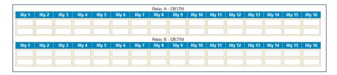
To assign a Netcue to a non-assigned relay, simply enter the 3-character Netcue code into the box below the target relay:
